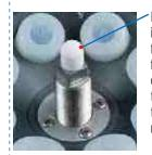
Rotor identification head, when the centrifuge lid is closed the rotor communicates all the data of the functions of it. This prevents, before use, any risk of failure of using the wrong rotor in a program or exceeding the rotors running parameters. The advantage of this system is that we can add additional rotors to the range without changing the centrifuge model
